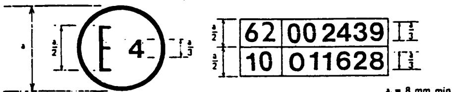
The above approval mark affixed to a vehicle shows that the vehicle type concerned has been approved in the Netherlands (E 4) pursuant to the Regulations Nos. 62 and 10.<sup>(1)</sup> The approval numbers indicate that, at the dates when the respective approvals were given, Regulation No. 62 had not been modified, and Regulation No. 10 already included the 01 series of amendments.
