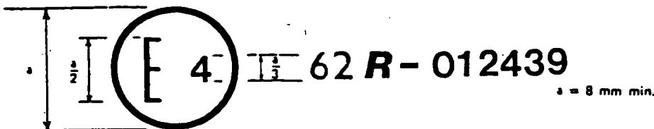
The above approval mark affixed to a vehicle shows that the vehicle type concerned has, with regard to the protection against unauthorized use, been approved in the Netherlands (E 4) pursuant to Regulation No. 62 under the approval number 002439. The approval number indicates that the approval was granted in accordance with the requirements of Regulation No. 62 in its original form.
